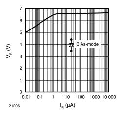
Fig. 5 - Typical Reverse Voltage V<sub>R</sub> vs. Reverse Current I<sub>R</sub>
