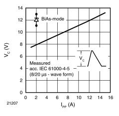
Fig. 6 - Typical Peak Clamping Voltage  $V_{C} \mbox{ vs.}$
