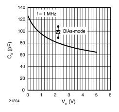
Fig. 3 - Typical Capacitance  $C_{\text{D}}$  vs. Reverse Voltage  $V_{\text{R}}$
